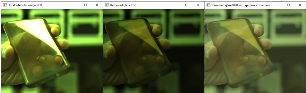
Figure 5 – The result of the application (left full intensity image, middle image with glare removed, right image with glare removed and gamma correction).
